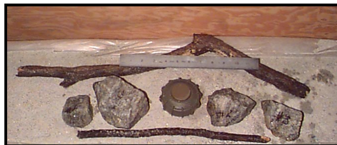
Photograph showing the relative size of the mine and the clutter objects.
