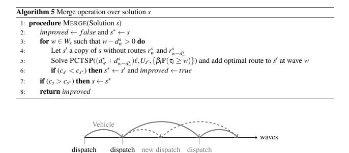
Figure 8: Example of an exchange operation where a dispatch gives one wave to its successor (dashed flow).
