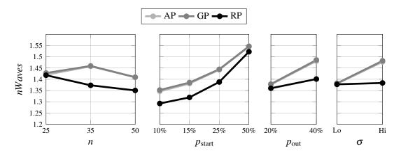
Figure 11: Average number of waves per vehicles dispatch versus n,  $p_{start}$ ,  $p_{out}$ , and  $\sigma$
