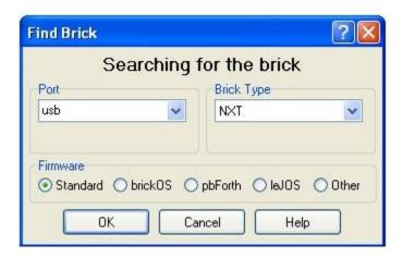
Select "Automatic" or "usb" under Port and "NXT" under Brick Type. Firmware should be set to "Standard" by default.
