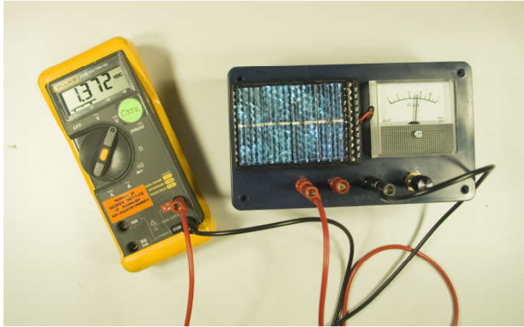
Figure 7: Solar panel experiment to measure I-V curves, on left, with resulting I-V curve, on right.
