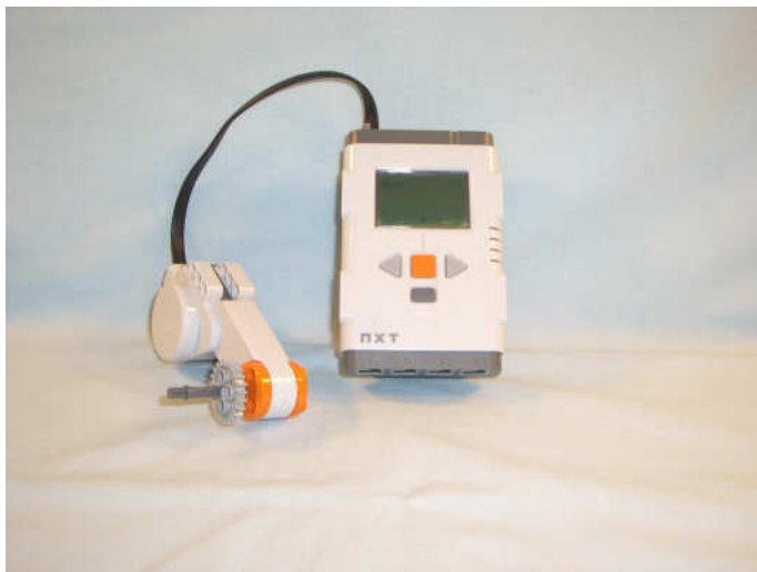
Figure 5: LEGO NXT motor control experiment. Students can enter a gain directly in the NXT processor interface and run the motor position controller with different levels of gains. They can try to turn the motor away from its set point and find that the higher the gain, the harder it is to turn the motor from its set point
