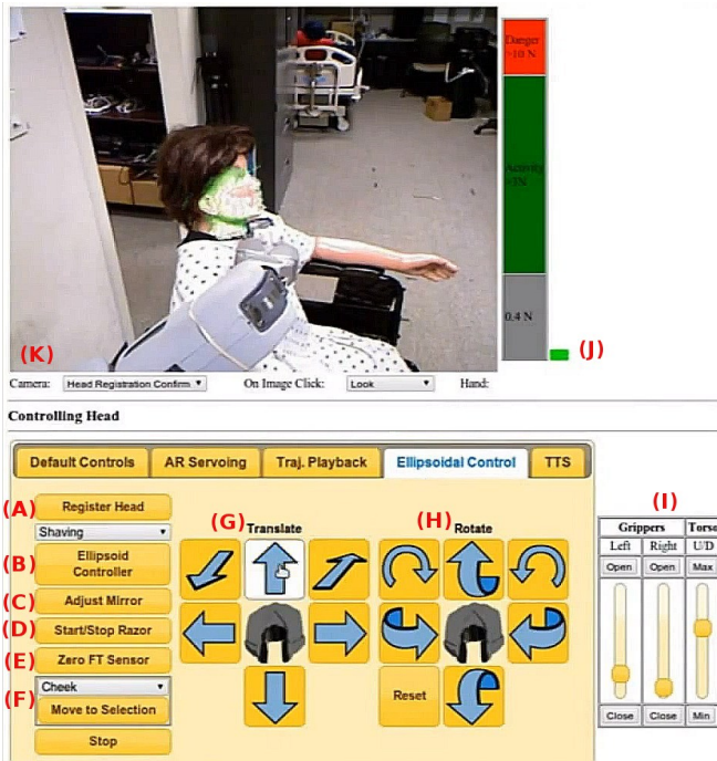
Fig. 6. Ellipsoidal Control Interface: (A) Begin head registration. (B) Activate ellipsoidal control. (C) Point mirror at head. (D) Toggle shaver power. (E) Re-zero force/torque reading. (F) Select head location for global movement . (G) Translate locally in E-space. (H) Rotate locally in E-space. (I) Control gripper and torso. (J) End-effector force display. (K) Live camera feed with registration confirmation overlay.
