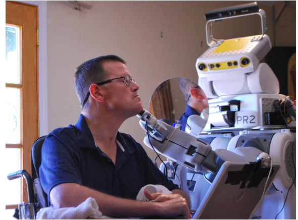
Fig. 1. Shaving Using a PR2 Robot: Henry Evans, a man with quadriplegia, using the PR2 robot to shave the left side of his face while he sits in his manual wheelchair in the living room at his home. He uses a head-tracking mouse on the laptop in front of him to operate the system. The robot is holding a mirror and an electric shaver.
