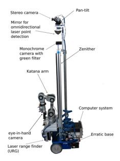
Fig. 2. An image of the assistive mobile manipulator El-E (pronounced "Ellie") used in this work. El-E has a 5-DoF arm (Neuronics Katana) on a vertical lift as well as a variety of sensors. In this work, El-E uses its gripper in a manner similar to the way a service dog uses its mouth. El-E also makes use of an eye-in-hand camera and force/torque sensors in its fingers.
