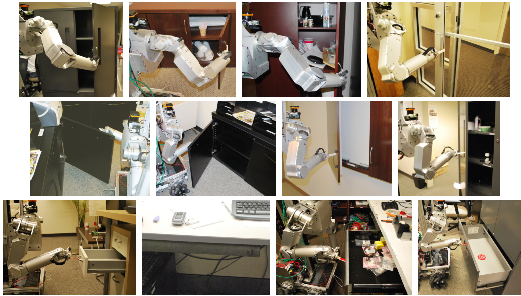
Fig. 10. Images showing the robot after it has operated 11 mechanisms with the Pull-Radial-Force controller. The image of the drawer without the robot is the mechanism for which the hook slipped off before the drawer opened. The order of the mechanisms matches the results presented in Table II
