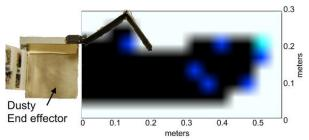
Fig. 7: Results of grasping a small cylindrical object at points on a grid. Black represents a grasping success rate of 3/3, dark blue represents 2/3, light blue represents 1/3, and white represents 0/3.
