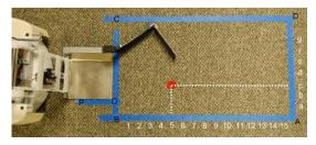
Fig. 5. Testing grasping area. Rectangle ABCD encircles the testing field. There are 7 markers on tape AD, and 15 markers on tape AB. The testing cylinder is placed on the mesh grids formed by these markers, e.g. the coordinate of cylinder shown in the figure is (5, c). Line BC and line OP are perpendicular to each other, and they define the starting position of the robot. The test is run with finger opened in the beginning.
