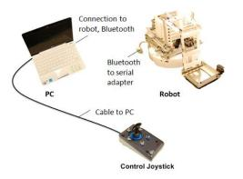
Fig. 2. For Dusty's user interface, joystick input is processed by the PC, which then transmits control information to the robot via Bluetooth.
