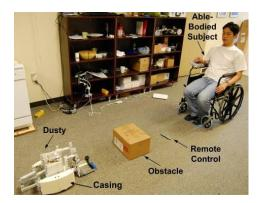
Fig. 6. **Experimental Setup:** Dusty (with protective casing) is in front of an able-bodied subject on a wheelchair, and an obstacle is placed in between the subject and the robot. The subject navigates the robot to avoid hitting the obstacle, fetches the remote control on the floor, and delivers it to himself.
