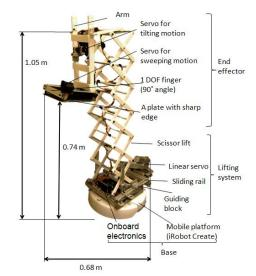
Fig. 3. Dusty consists of a mobile base, a lifting system, and an end effector
