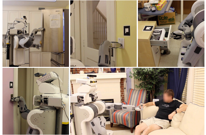
Fig. 1. Examples of robot behaviors constructed using the ROS Commander system and encapsulated as HFSMs: opening a fridge, unlocking with a button, opening a drawer, flipping a light switch, handing off an object.
