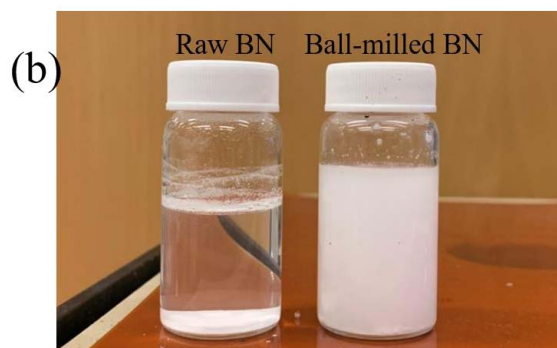
Fig 2. (a) FTIR spectra of raw and ball-milled BN and (b) picture of water-dispersed raw and ball-milled BN after settled for 30 minutes.
