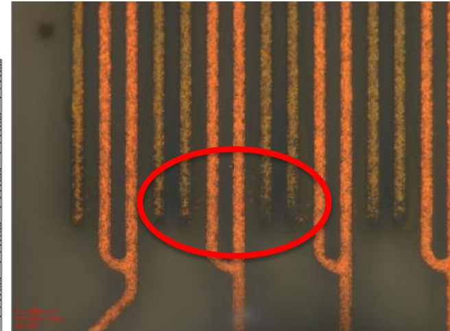
ECM failure in 1.5 \mu\text{m} space polymer RDL (0.6 wt.% moisture absorption)
