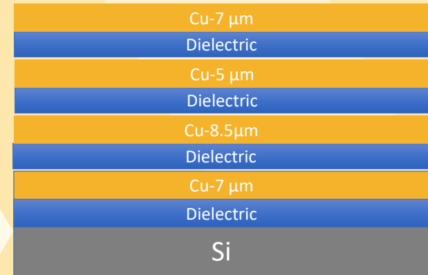
Schematic stack up of dummy ML RDL
