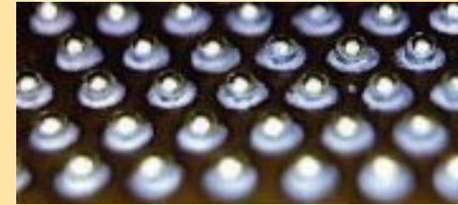
Complete wicking of solder paste on coated spheres
