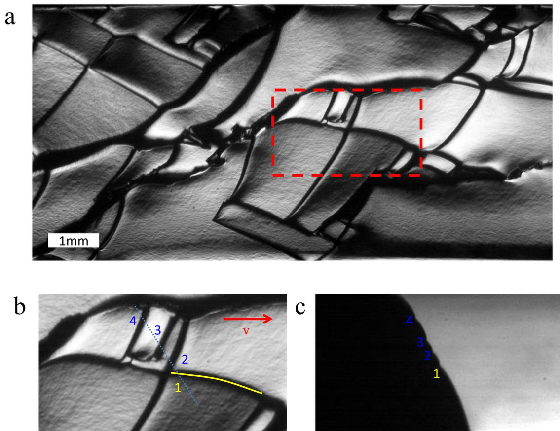
*Supplementary Figure 3. Dependence of step-line direction on the normal to the crack front.* (a) A typical fracture surface in the faceting regime. (b) A section of a fracture surface in (a) with a step-line extending nearly parallel to the X axis highlighted in yellow. Numbers refer to curved points along the front in (c). The dotted light blue line approximates the front tilt in (c). (c) A snapshot of the crack front that created the surface in (b) reveal strong tilting of the front.
