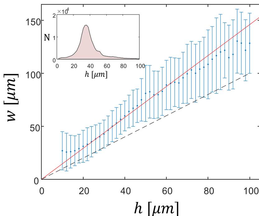
*Supplementary Figure 2. Step width  $w$  grows with step height  $h$ .* Blue bars show the range of  $w$  measured by profilometry when averaged over  $2\mu\text{m}$  intervals of  $h$ . Linear regression (red line) yields a proportionality coefficient of  $1.4 \pm 0.4$ . The dashed black line,  $w = h$ , is one standard deviation below the mean. (*inset*) Number of data points within each  $2\mu\text{m}$  interval of  $h$ . A total of  $\sim 155,000$  points was considered.
