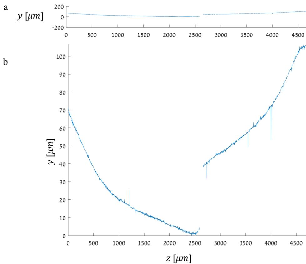
*Supplementary Figure 4.* (a) The height profile along the  $z$  axis of a fracture surface containing a single step (at  $z \sim 2500\mu\text{m}$ ) taken at a constant  $x$ . Except at the step, surface height barely changes, and the wavelength of its variation is of the order of the sample thickness ( $\sim 4.6\text{ mm}$ ). (b) The same height profile with the  $y$  axis blown-up by a factor of 45.
