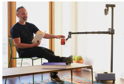
Fig. 1. The Stretch RE1 from Hello Robot Inc. teleoperated to hand an object to Dr. Aaron Edsinger in a real home.
