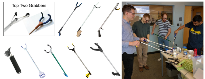
Fig. 4. Left : Amazon product images for the ten grabbers we evaluated at Georgia Tech in May of 2017. The inset shows the top two. We converted the top left grabber into a robotic gripper. Right : Members of the Healthcare Robotics Lab evaluate grabbers by manipulating objects relevant to assistive robotics, including a pill and a utensil [61].
