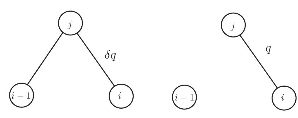
The left graph edge (i - 1, j) is present, the probability of generating (i,j) is  $\delta q$  where q:= $P\{X_i^{(j)} = 1\}$  and  $X_i^{(j)}$  is the variable of edge (i-1,j).
