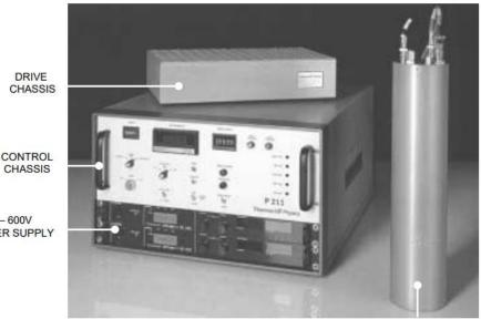
NTTA NEUTRON TUBE AND TRANSFORMER ASSEMBLY
