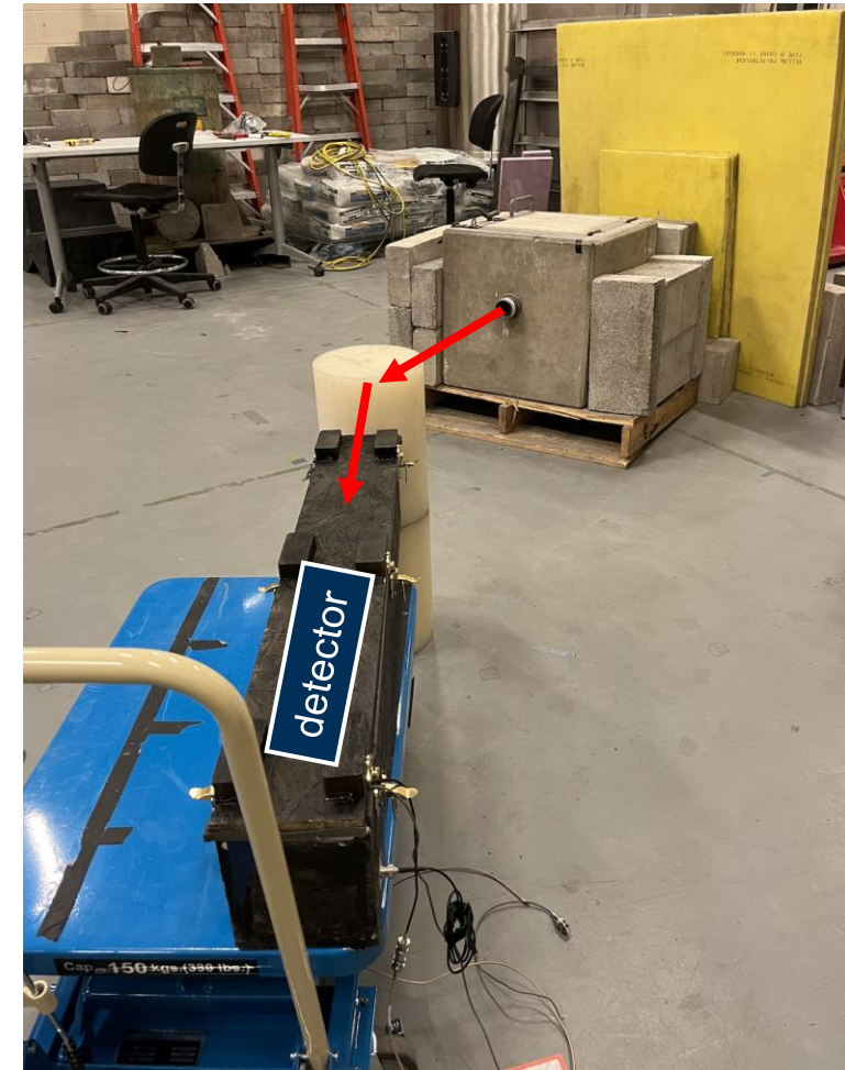
AmBe setup: Poly, concrete, water, 3" lead to knock down gammas
