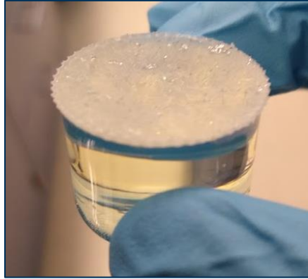
Dopant Precipitation on Surface
