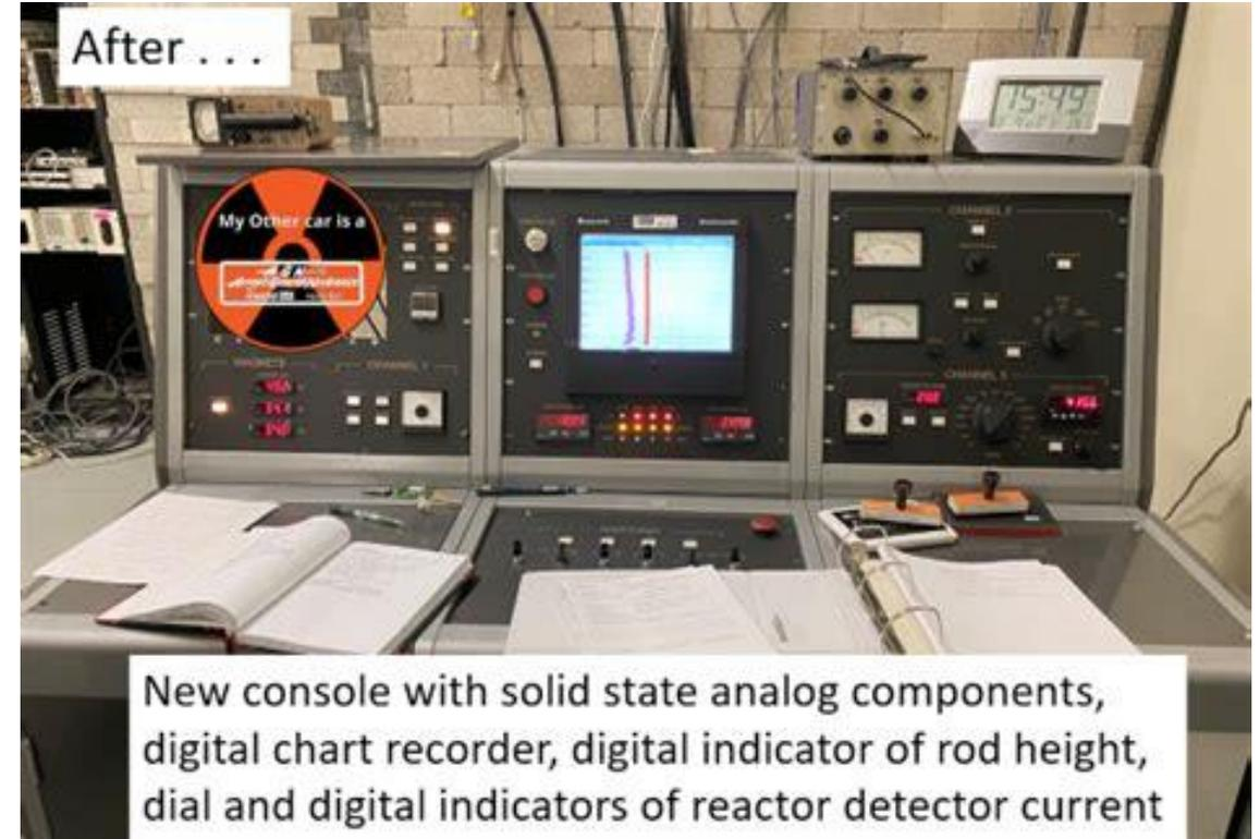
New console with solid state analog components, digital chart recorder, digital indicator of rod height, dial and digital indicators of reactor detector current
