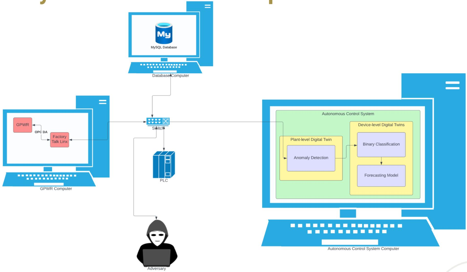
In this scenario, the reactor is “air-gapped” from unsecured networks, meaning the adversary must have physical access to the system to launch attacks.
