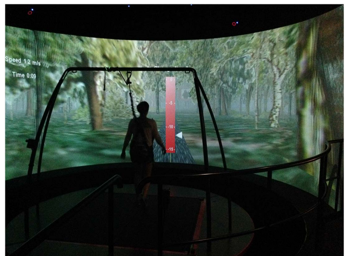
Figure 1 — Virtual environment with biofeedback display: an arrow moved continuously along the vertical scale displaying the step-by-step vertical ground reaction impulse (vGRI) of the target limb (as a percentage relative to previously recorded baseline vGRI at a given speed). Values were reflective of the prior step of the target limb.
