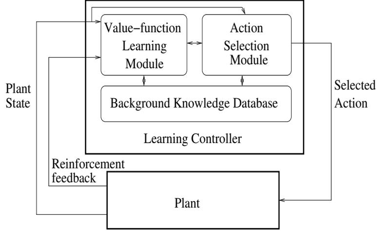
Figure 3: The basic architecture of a RL-based controller
